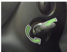
Turn the ignition key to the "OFF position" and remove it
